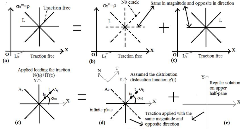
FIGURE 3.1. (a) The original problem,  $\sigma_x^\infty = p$ , (b) An elastic half-plane,  $\sigma_x^\infty = p$ , (c) A branch crack with the applied loading, (d) A branch crack in an infinite plate, (e) The upper half-plane's regular solution.
