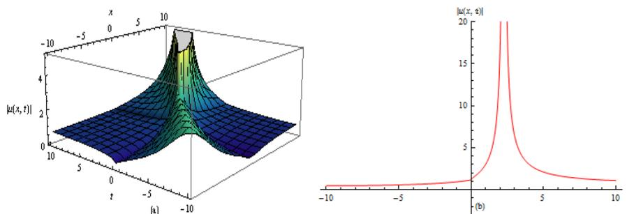
FIGURE 9. (a) Three dimensional plot for singular soliton solution of (5.28) where  $\lambda = 0.5, \mu = 0, \gamma = -1, c = -1, c_2 = 1, c_3 = 1, \alpha = 0.5, \nu = 1$  (b) Two dimensional line plot of (5.28) with  $t = 1$ .
