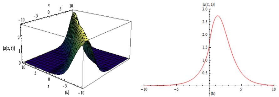
FIGURE 4. (a) Three dimensional plot for dark soliton solution of (5.16) where  $\lambda = 3, \mu = 2, \gamma = 1, c = -1, c_2 = -1, \alpha = 0.8, \nu = 1$  (b) Two dimensional line plot of (5.16) with  $t = 1$ .
