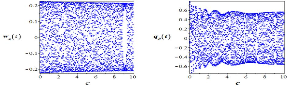
FIGURE 4. Bifurcation diagrams corresponding to angular velocity  $w_z$  and quaternion parameter  $q_2$  under torques  $c_x = c_y = c_z = c \in [0, 10]$  of the system (2.4) and (2.5).
