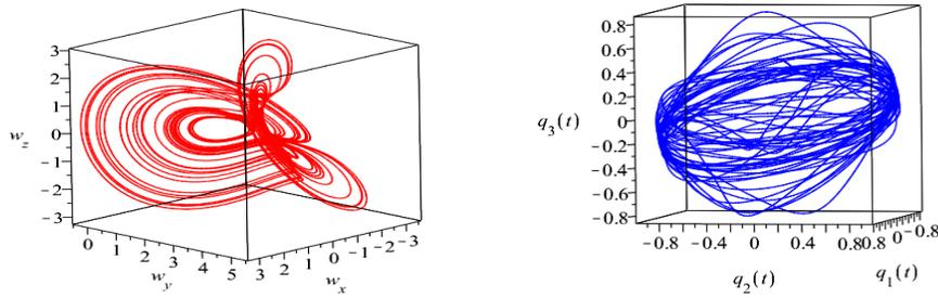
FIGURE 2. Phase portraits of the angular velocities and quaternion parameters of SA system, whit perturbing torque (3.1).
