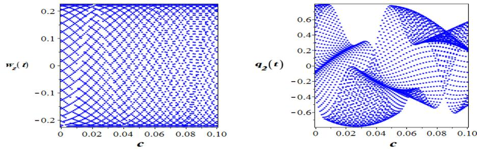
FIGURE 5. Bifurcation diagrams corresponding to angular velocity  $w_z$  and quaternion parameter  $q_2$  under torques  $c_x = c_y = c_z = c \in [0, 0.1]$  of the system (2.4) and (2.5).
